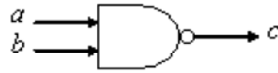
Fig.1: Schematic diagram of the NAND gate which has the following truth table
