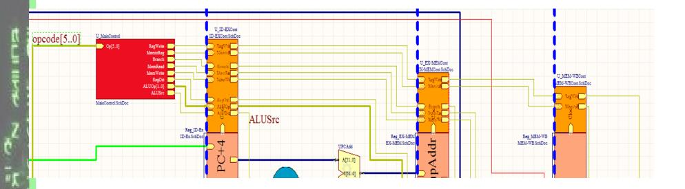
Outputs travel between registers and are wired to correct datapath unit at the appropriate instruction stage
