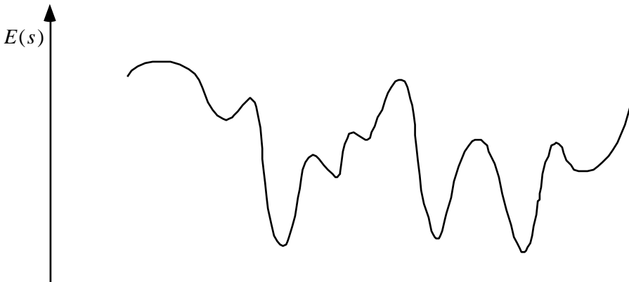
Figure 1.7.4 Schematic plot of a system energy E(s) as a function of a system coordinate s . In simulated annealing, the location of a minimum energy is sought by starting from a high temperature Monte Carlo and cooling the system to a low temperature. At the high temperature the system has a high kinetic energy and explores all of the possible configurations. As the temperature is cooled it descends into one of the wells, called basins of attraction, and cannot escape. Finally, when the temperature is very low it loses all kinetic energy and sits in the bottom of the well. Minima with larger basins of attraction are more likely to capture the system. Simulated annealing works best when the lowest-energy minima have the largest basins of attraction. ■
