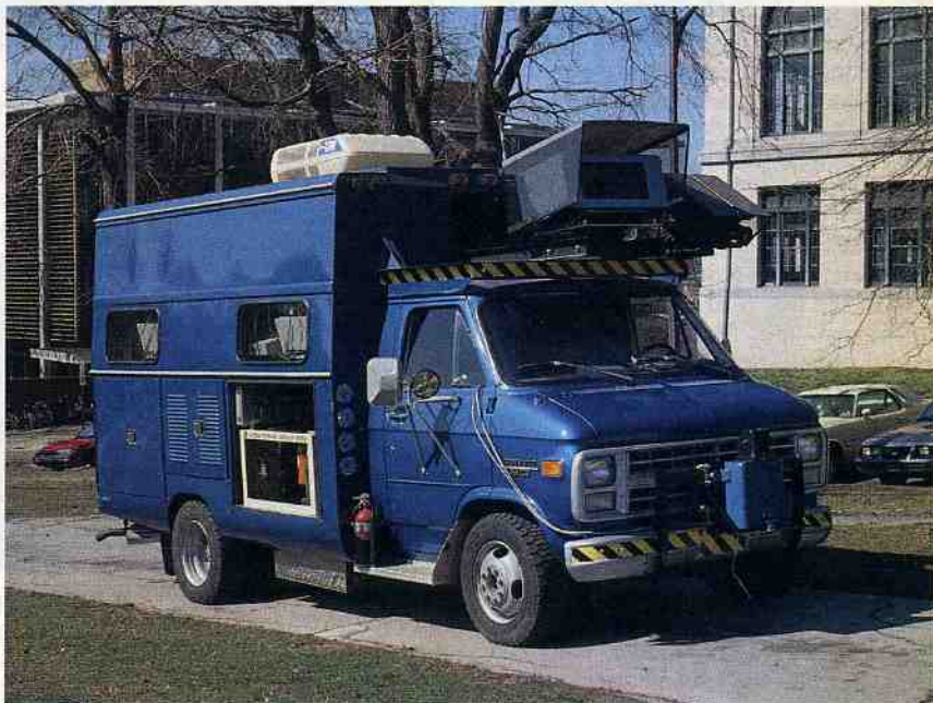
Photo 1: The NAVLAB autonomous navigation test-bed vehicle and the road used for trial runs.
