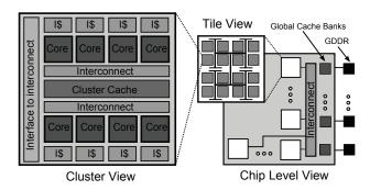
Figure 2: Diagram of the Rigel processor.
