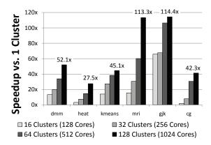
Figure 5: Speedup of one, two, four, and eight (1024 core) tile configurations over execution on a single 8-core Rigel cluster. There are sixteen clusters (128 cores) per tile.
