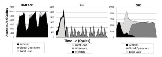
Figure 6: Three global cache traffic patterns from: kmeans, where atomic operations dominate the global cache traffic due to a histogram optimization; cg, where writebacks of shared data dominate, but do not saturate the global cache bandwidth; and gjk, showing high levels of load balancing resulting in global task queue actions dominating global cache traffic. With additional tuning we have found most of this overhead can be removed.
