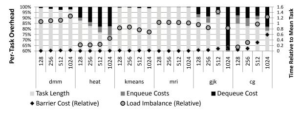
Figure 7: The per-task cost of task execution, barriers, enqueue, and dequeue operation are plotted as a percentage of the average task length in cycles.
