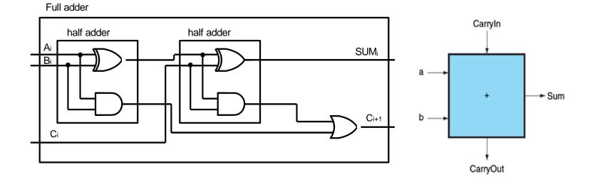
Note: A full adder adds 3 bits. Can also consider as first adding first two and then the result with the carry
