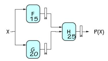
Now F & G can be working on input X<sub>i+1</sub> while H is performing its computation on X<sub>i</sub>. We've created a 2-stage *pipeline*: if we have a valid input X during clock cycle j, P(X) is valid during clock j+2.
