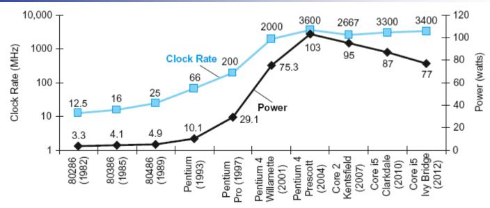
Clock rate and Power for Intel x86 microprocessors over eight generations
