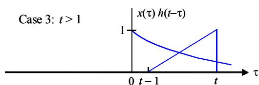
Figure Q1: Convolution of the input signal  $x(t)$  with the impulse response  $h(t)$ .
