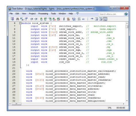
Figure 7. A part of the generated Verilog module.
