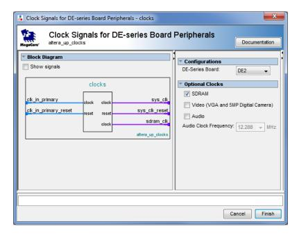
Figure 11. Clock Signals IP Core
