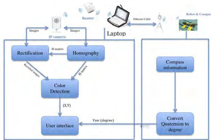
Fig. 6: Block diagram of the system showing the interactions between nodes
