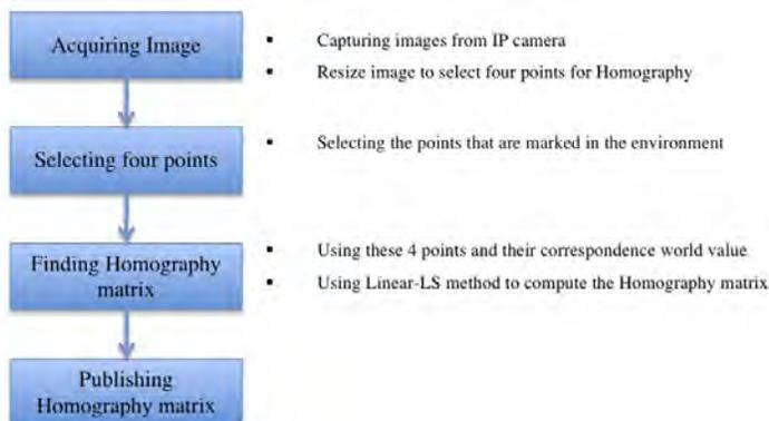
Fig. 7: Flowchart to determine homography matrix for every camera
