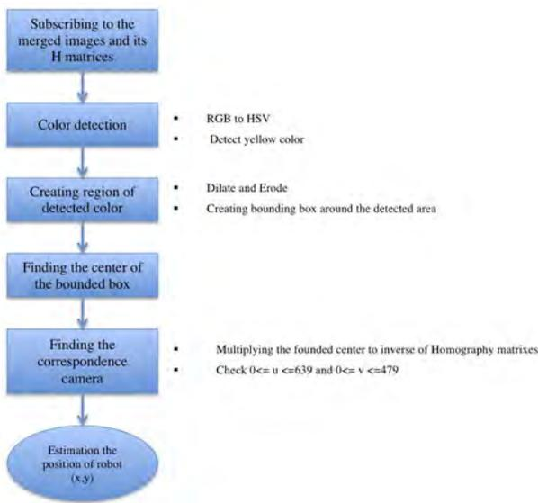
Fig. 9: Flowchart to detect the Kingfishers pontoons (yellow colour) and determined the position of the robot
