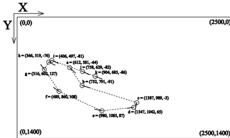
Fig. 11: Simultaneous position and orientation results at specific locations of the robot shown on the plan view of the pool. The numbers shown for each point are x coordinate (cm), y coordinate (cm), and rotation (degree) respectively
