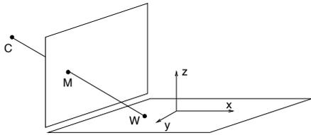
Fig. 3: The map between a world plane and a perspective image is an homography
