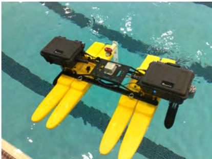
Fig. 13: The LED mounted at an specific height on the Kingfisher used as the first target
