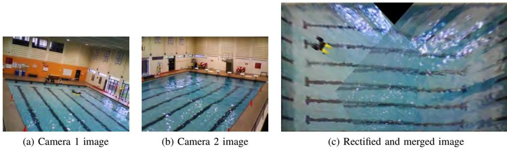
Fig. 8: Rectification and merging of the camera images
