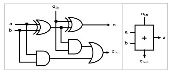
We now like to use abstraction to encapsulate this functionality. To that end, we repackage the adder as a component named <code>yAdder1</code> and having the block diagram shown in the right part of the figure (it operates on 1-bit wires and thus the 1 suffix).
