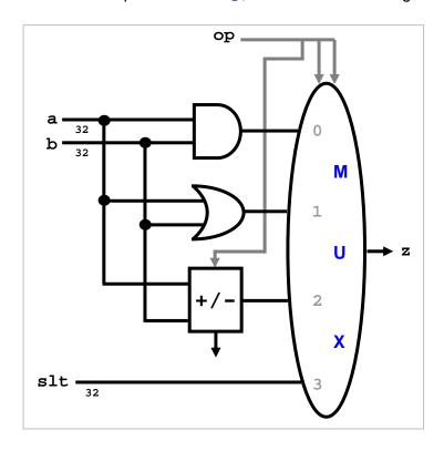
As you can see in the diagram, we used the most significant bit of op, i.e. op[2], as a control signal for the adder / subtractor. The other two bits, i.e. op[1:0], are used to control the mux—to select the component whose output is to emerge as the output of the ALU.
