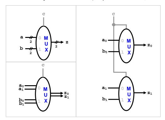
The right side of the figure shows how to build yMux2 using two yMux1's.
