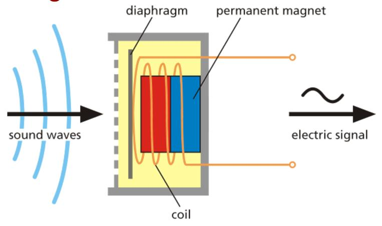
Sound waves travelling through the air hit the diaphragm
